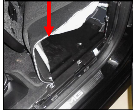
Fold up flooring, disassemble plastic cover
